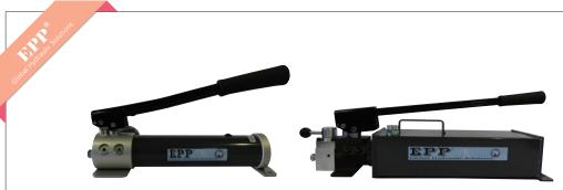
Reservoir Capacity: 350-7800cc Flow at Rated Pressure: 0.82-4.75cc/stroke Maximum Operating Pressure: 700 BAR
